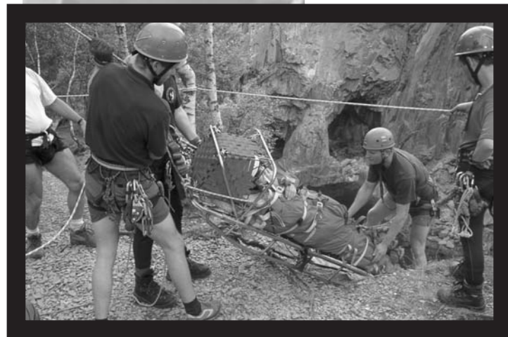
Peter Bell magnanimously volunteered to be casualty in his own stretcher – a new, lightweight design which still exhibits the massive strength people expect of a Bell stretcher. This vertical orientation was more to test the head yoke and lowering/belay than an indication of normal procedure.
