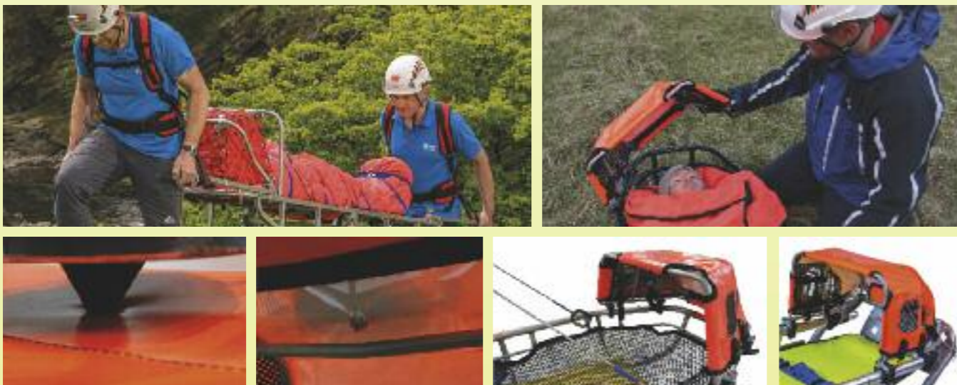
Clockwise from below: Bell head guard 'in action'; Open head guard; Mark 6 Head guard; Basket head guard; Spike test impact internal; Spike test impact external. Opposite page: Test set.
